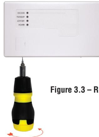
Figure 3.3 – Removing Cover
